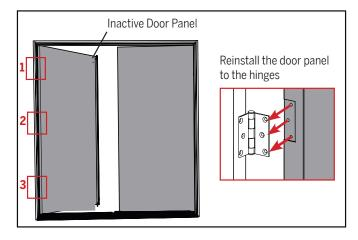
a. Reinstall the inactive door panel by screwing the door panel back to the hinges.
