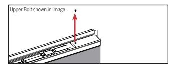
b. Secure the bolt sleeve by installing the screw.
