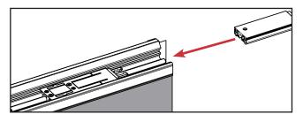
a. Slide the bolt sleeve onto the shoot bolt in the astragal body.
