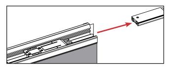
b. Slide the bolt sleeve out of the astragal body.
