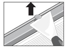
1. Pry off the old cap plugs from the sill cap using a putty knife, flathead screwdriver or similar tool.
