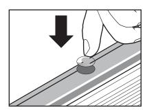
2. Install the replacement cap plug by centering it over the cap hole and pressing it down firmly until it snaps into place.
