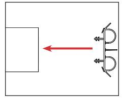
b. Orient the door bottom with the door panel as shown above.
