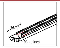
c. Cut the kerf legs, where they meet the door bottom until they are removed. Be sure to cut the kerf legs as close to the door bottom as possible to ensure a flat surface.
