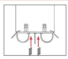
c. Complete insertion by moving along the length of the door bottom. Secure each end with a 1/2" x 1/2" light gauge staple. Wipe away excess caulking.
