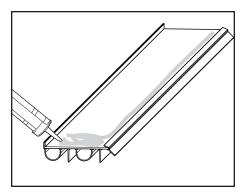
a. Apply exterior grade caulking along the edge of the door bottom that will be facing the exterior of the home. Thoroughly caulk each end of the door bottom.
