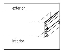
a. Align one end of the door bottom with the door panel edge on the lock side.
