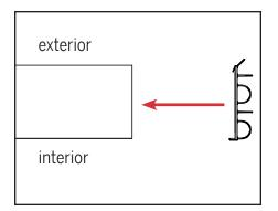
b. Orient the door bottom with the door panel as shown above.
