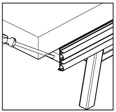
a. Remove the old door bottom from the door panel. Use a flathead screw driver to pry the end of the door bottom off the panel.
