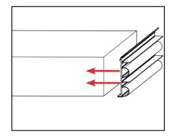
b. Using hand pressure, press the door bottom flush against the bottom of the door panel. Make sure the door bottom is flush down the length of the panel and square at the ends.
