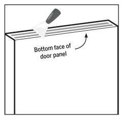
b. Remove any old residue or staples from the door panel's bottom face, using a putty knife or similar tool.
