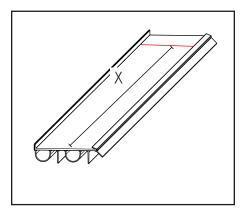
b. Measure and mark the same width (X) on the door bottom, measuring from one end. Cut the door bottom along that line.
