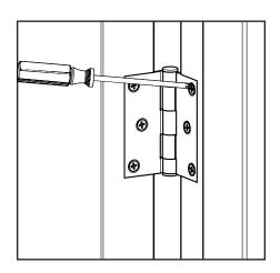
a. Open the door and locate the hinges. Using a Phillips screwdriver or drill, remove the screws from the hinge plate on the jamb.
