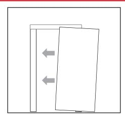
a. Realign the door panel with the hinges in the frame.
