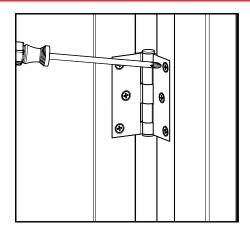
b. Reattach the hinges to the jamb with the screws previously removed. Confirm the door operates properly.
