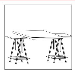
b. When door is loose from frame, carry it to a flat workspace where the panel can be laid horizontally.
