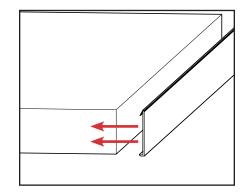
b. Using hand pressure, press the door bottom flush against the bottom of the door panel. Make sure the door bottom is flush down the length of the panel and square at the ends.
