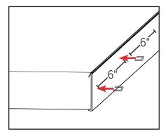
c. Secure one end with a 1/2" x 1/2" light gauge staple. Continue stapling down the length of the door panel in 6 inch increments. Wipe away excess caulking.
