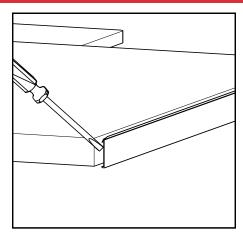
a. Remove the old door bottom from the door panel. Use a flathead screw driver to pry the end of the door bottom up.
