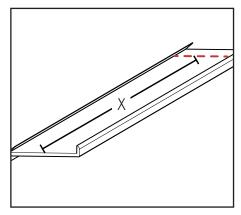
b. Measure and mark the same width (X) on the door bottom, measuring from one end. Cut the door bottom along this line.
