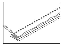
a. Apply exterior grade caulking along the edge of the door bottom that will be facing the exterior of the home. Thoroughly caulk each end of the door bottom.
