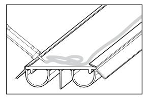
a. Apply exterior grade caulking along the edge of the door bottom that will be facing the exterior of the home. Thoroughly caulk each end of the door bottom.
