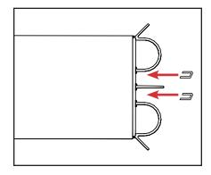
c. Secure one end with a 1/2" x 1/2" light gauge staple. Continue stapling down the length of the door panel in 6 inch increments. Wipe away excess caulking.
