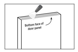
b. Remove any old residue or staples from the door panel's bottom face, using a putty knife or similar tool.
