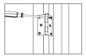
a. Open the door and locate the hinges. Using a Phillips screwdriver or drill, remove the screws from the hinge plate on the jamb.
