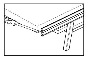
a. Remove the old door bottom from the door panel. Use a flathead screwdriver to pry the end of the door bottom off the panel.
