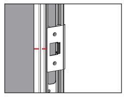
a. Place the plates against the retainer, being sure to center the plate with the mark you made in Step 3.
