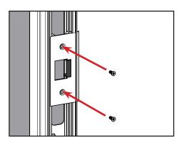
b. Screw in the strike plate to secure them on the retainer. Repeat for all strike plate locations.
