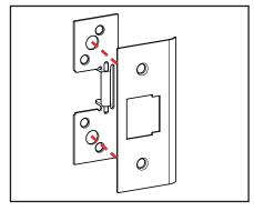
a. Attach the reinforcing plate to the strike plate by aligning the screw holes.
