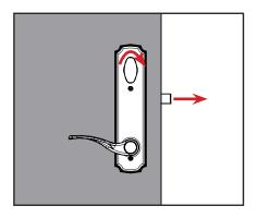
a. With the door slightly open, turn the Trilennium® lock to engage the deadbolts.
