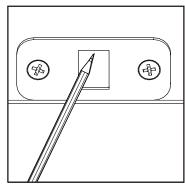
a. Trace the rectangular space of the strike plate with a pencil to use as a template to drill the holes.
