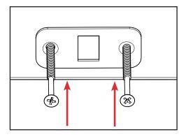
b. Spot drill the location of the screw holes. Once spot drilled, fully secure the plate into the header temporarily with the screws provided.
