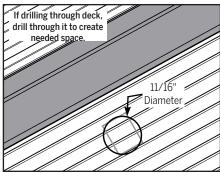
c. Drill into the sill cap or deck using an 11/16" diameter drill bit to create a space at least 1" deep.
