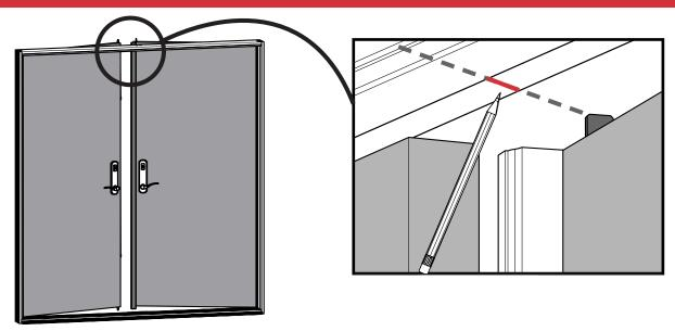
Close the inactive door and engage the bolts. Mark the area where the lock will meet the header. This will serve as a reference point to mount the strike plate.
