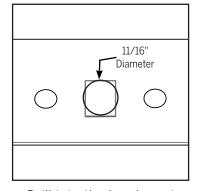
c. Drill into the header using an 11/16" diameter drill bit to create a space at least 1" deep.
