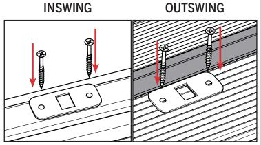
b. Spot drill the location of the screw holes. Once spot drilled, fully secure the plate into the sill with the screws provided.
