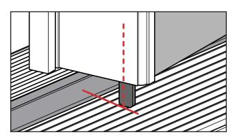
Close the door until the length of the door panel is parallel to the sill cap. Mark the centerline of the door panel onto the sill deck.
