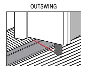
Close the inactive door and turn the lock to engage the upper and lower bolts. Mark where the lock meets the sill cap or deck. This will serve as a reference point to mount the strike plate.
