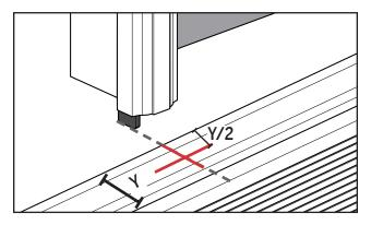
Measure the width of the sill cap (Y) and mark the center point (Y/2).
