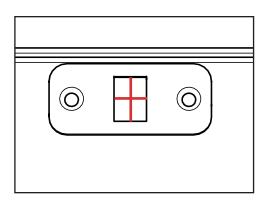
a. Using the marks you have made in Steps 1 and 2, line up the strike plate on the header.
