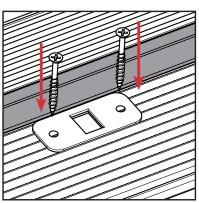
Return the strike plate to the exact position it was before (Step 9 & 10) and screw into place.
