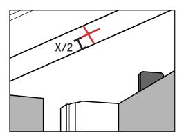
b. Divide this thickness (X) in half and mark that distance on the header. This will help you center the plate.
