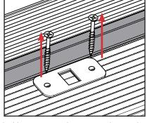
b. Unscrew and remove the strike plate.
