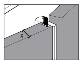
a. Measure the thickness of the door panel (X).
