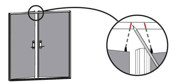
Close the inactive door and turn the lock to engage the upper and lower bolts. Mark where the lock meets the header. This will serve as a reference point to mount the strike plate. Repeat this with the active door panel.
