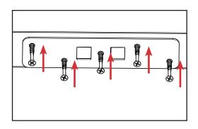
**Note:** You will only be able to confirm proper installation of the header strike plate after you install the strike plate on the sill and are able to fully close the door. Proceed to Part B for sill strike plate installation.
