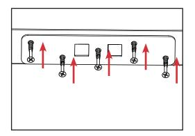
b. Spot drill the location of the screw holes. Once spot drilled, fully secure the plate temporarily into the header with the screws provided.
