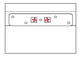
a. Using the marks you have made in Steps 1 and 2, line up the strike plate on the header.
