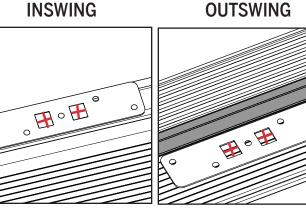
a. Using the marks you have made in Steps 7 and 8, line up the strike plate on the sill cap or deck.
