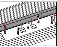
b. Unscrew and remove the strike plate.
