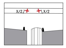
b. Divide this thickness (X) in half and mark that distance on the header. This will help you center the plate.
