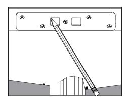
a. Trace the rectangular space of the strike plate to use as a template to drill the needed holes.
