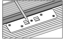
a. Trace the rectangular space of the strike plate with a pencil to use as a template to drill the holes.
