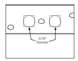
c. Drill into the header using an 11/16" diameter drill bit to create a space at least 1" deep.
