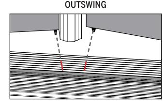
Close the inactive door and turn the lock to engage the upper and lower bolts. Mark where the lock meets the sill cap or deck. This will serve as a reference point to mount the strike plate. Repeat this for the active door.
