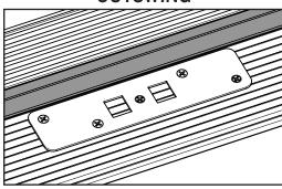
Return the strike plate to the exact position it was before (Steps 9 & 10) and screw into place.
