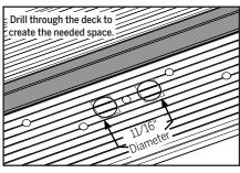
c. Drill into the sill cap or deck using an 11/16" diameter drill bit to create a space at least 1" deep.
