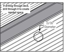
c. Drill into the sill cap or deck using an 11/16" diameter drill bit to create a space at least 1" deep.
