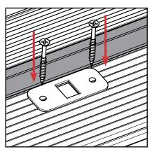
Return the strike plate to the exact position it was before (Steps 9 & 10) and screw into place.
