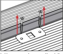
b. Unscrew and remove the strike plate.
