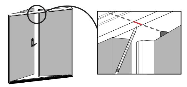
Close the inactive door and engage the magnum bolts. Mark where the lock meets the header. This will serve as a reference point to mount the strike plate.
