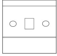
b. Unscrew and remove the strike plate.
