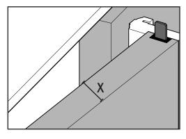
a. Measure the thickness of the door panel (x).
