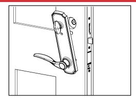
b. Carefully remove the plates from the door panel.
