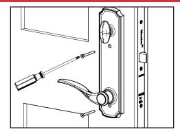
a. Remove the 2 mounting screws on the interior handset that are securing both plates together.
