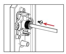
c. Secure the cylinder using the tapping screw you removed in step 2.
