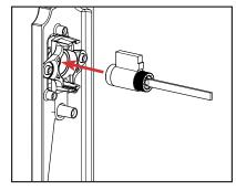
b. Insert the key cylinder into the upper hole from the back side of the faceplate with the tab pointing up.
