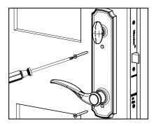
d. Secure the handsets with the mounting screws from the interior to exterior. Do not overtighten.
