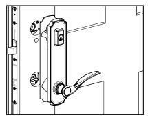
b. Start with the exterior handset. If the gasket is still present, align it with inside face of the faceplate. Guide the cylinder tailpiece and handle cartridge into the respective hubs on the lock hardware. Hold in place.
