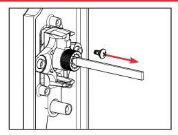
a. Remove the screw securing the current key cylinder.
