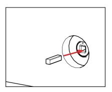
a. If the square spindles fell out of the lock when the faceplates were removed, reinsert them into their hubs within the lock.
