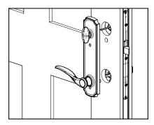
c. With the interior handset, guide the thumb-turn receiving slot towards the cylinder tailpiece and align the handle cartridge with the spindle. Both handsets should lay flush against the door panel.
