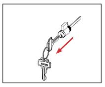
a. Remove the keys from the key cylinder.
