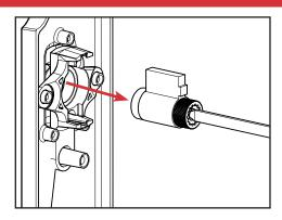
b. Remove the key cylinder from the handset faceplate.
