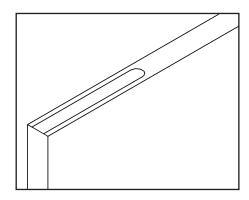
c. Check that the traced outline is centered on the door and flush with the end.
