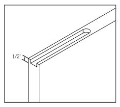
a. Use a router with a 1" diameter bit to create the groove within the lines you traced in the previous step.
