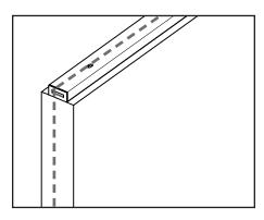
b. Center the bolt along the width of the door and trace around the bolt.
