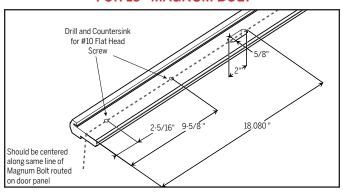
a. Prepare the astragal with the holes shown above to allow for Magnum Bolt access.
