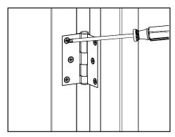
a. Loosen screws at the hinges on the door panel. Repeat on other hinges. Set the door with the hinge side down and clamp it to something to give you a stable work surface.
