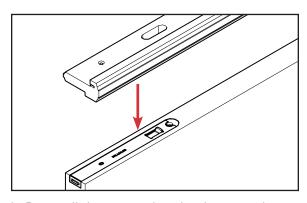
b. Reinstall the astragal to the door panel, over the Magnum Bolt. Confirm the holes on the astragal provide proper access to the Magnum Bolt.
