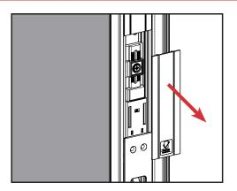
Remove the existing actuator cover off the astragal on the inactive door, using pliers if necessary.
