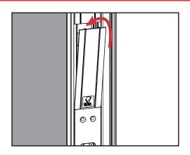
Place new actuator cover with the logo on the bottom and snap into place. Return surrounding trim strip in place, if previously removed.
