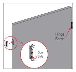
a. Insert the assembly into each pocket as shown. The open side of the keeper may face barrel of hinge when installed.
