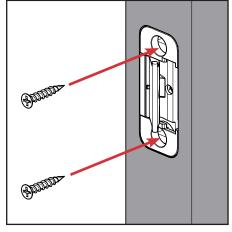
b. Secure each assembly with (2) #8 x 1" screws.
