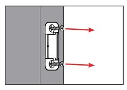
Remove the two screws from the keeper and pull the assembly out of the pocket.
