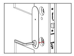
a. Place the interior handset onto the door, with the handle end aligning into the hub in the Trilennium lock.
