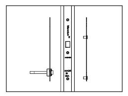
b. Align the exterior handset on the outside of the door panel. The screw bosses should fit into the door holes.
