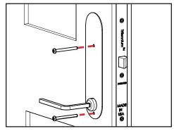
a. Secure the plates in place using the #10-32 machine screws provided.
