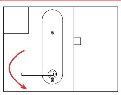
b. Once installed, ensure the handle operates the latch.
