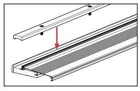
b. Replace the sill cap by screwing into place. Tighten the screws incrementally along the cap for a uniform reinstallation.
