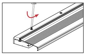
a. Remove the wood sill cap by gradually loosening the screws across the length of the sill. Remove and set aside
