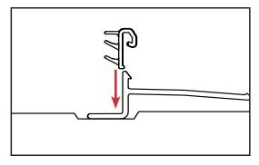
a. Replace with new rainseal gasket ensuring that it sits securely along the sill dam.
