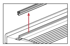
b. Remove the existing rainseal gasket from the sill dam, if present.
