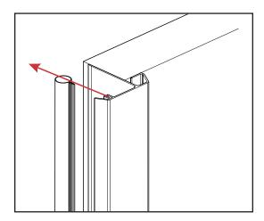
b. Remove the old weatherstrip, using the needle nose pliers if necessary. At this point, clean the kerf slot thoroughly before placing new weatherstrip.
