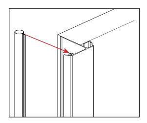
Starting at the top, work your way down the security flange, firmly pressing the weatherstrip into the kerf slot.
