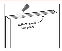
b. Remove any old residue or staples from the door panel's bottom face, using a putty knife or similar tool.
