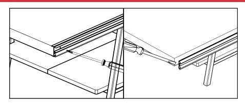
a. Remove the old door bottom from the door panel by removing the screws, if it was a screw-on door bottom. If the door bottom was staple-on, you may need to pry it off with a flathead screwdriver.
