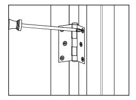
a. Open the door and locate the hinges. Using a Phillips screwdriver or drill remove the screws from the hinge plate on the jamb.
