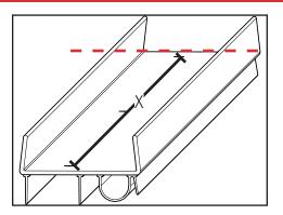
b. Measure and mark the same width (X) on the door bottom, measuring from one end. Cut the door bottom along that line.
