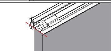
When the bolt is in the unlocked (retracted) position, the end of the bolt must be flush with the end of the astragal.
