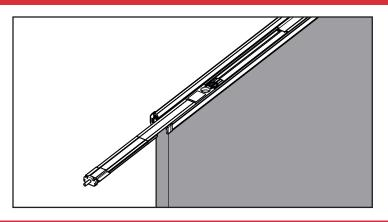
Slide the bolt you wish to replace out of the astragal using the finger notch on the bolt. (Lower bolt shown in image).
