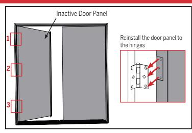
Reinstall the inactive door panel by screwing the door panel back to the hinges.
