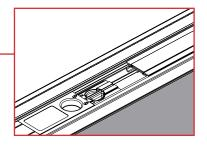
Slide the new flush bolt into the astragal and under the strike support.
