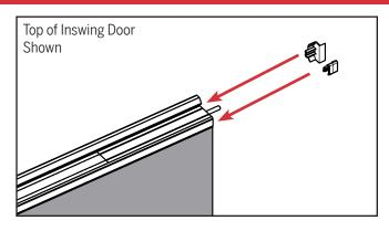
b. Install the trim cap and spacer to the top.
