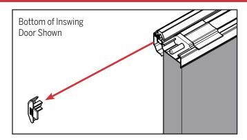
a. Remove the trim cap from the bottom of the astragal. If outswing, remove the spacer.
