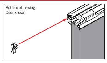
a. Install the new trim cap to the bottom of the astragal. For outswing doors, install the new spacer to the bottom as well.
